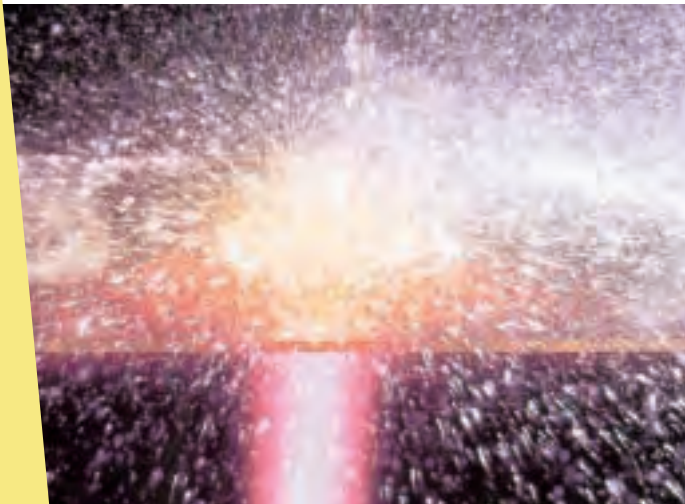
The thermal expansion coefficient of FireLite is almost 'zero' so it will not crack when heated to 800°C and then hit with cold water. FireLite is manufactured by Nippon Electric Glass Co. Ltd. Japan
