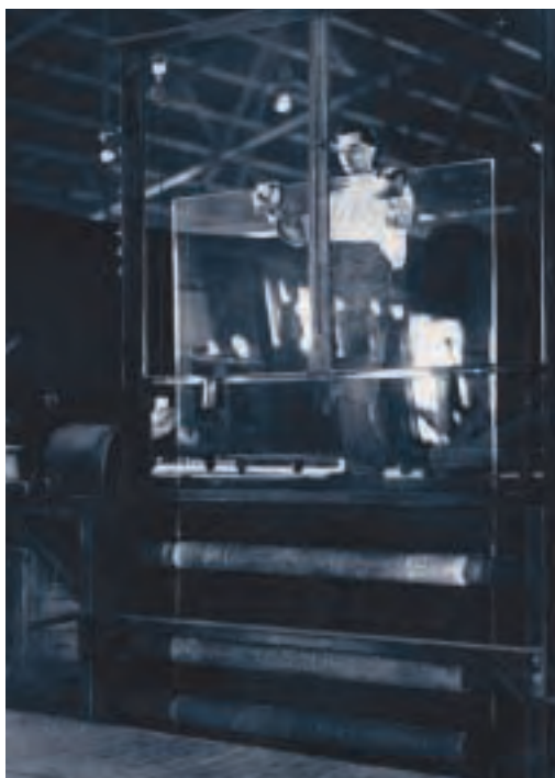
The Fourcault process in action
