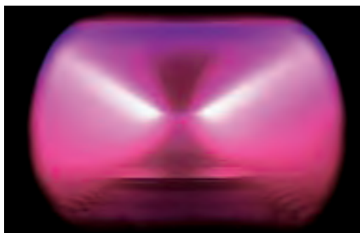
Plasma glow during the sputtering process
